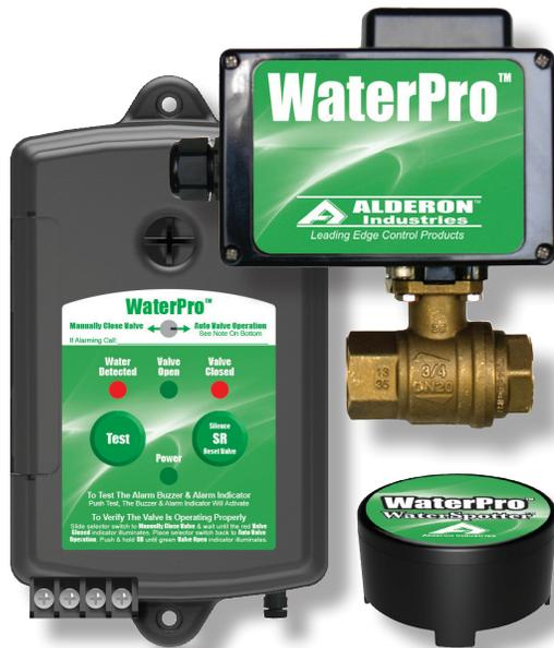
The WaterPro™ V-Series Valve Control system is an indoor rated alarm panel, powered by a standard 120VAC wall outlet. When powered, the green LED will illuminate on the alarm panel. Included with the system is a WaterPro™ WaterSpotter™ Flood Sensor and a lead-free full-port WaterPro™ Motorized Ball Valve (ranging in sizes from 1/2" to 1 1/4" NPT thread).
