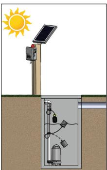
Must be installed in location with adequate sunlight for solar charging. Unit in full alarm without any solar charging will run for approximately 24 hours.
