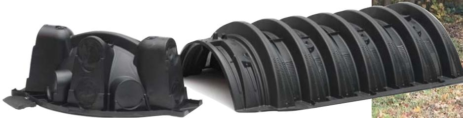
The Quick4<sup>®</sup> Standard Chamber fits in a 36" wide trench and is ideal for curved or straight systems. It features the patent-pending Contour Swivel Connection<sup>™</sup> which permits turns up to 10°, right or left. The MultiPort<sup>™</sup> endcap allows multiple piping options and eliminates pipe fittings. The chamber's four-foot length provides optimal installation flexibility.
